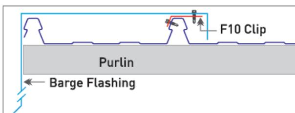
**Note:** This clip is positively fixed. Care should be taken when detailing industrial-length sheeting and flashing due to thermal expansion.
