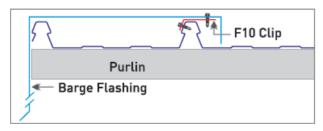
**Note:** This clip is positively fixed. Care should be taken when detailing industrial-length sheeting and flashing due to thermal expansion.
