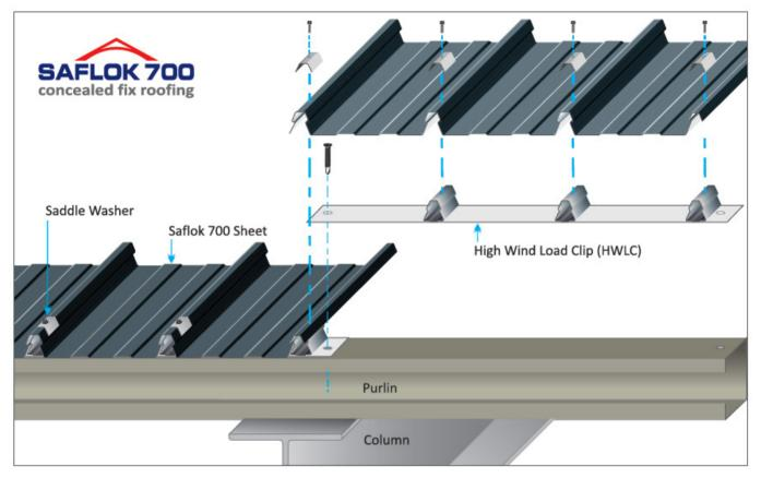
**Step 1.** Starting with the female rib first, align first sheet and hold down.
